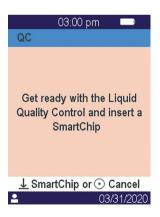
Refer to the instructions for use of the LQC to prepare the sample before inserting the SmartChip corresponding to the quality control to be performed. When the sample is ready, proceed in the same was as if it was to perform a routine test.
