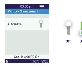
When automatic memory management is deselected, a new option called « Results deletion » is made available as part of submenu « Measurements ». This option allows to delete older results starting from the oldest one by using the navigation buttons.
