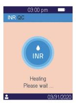
After heating, operator is prompted to drop a couple of drops of LQC on the curved plate of the Tsmart® to perform the quality control test:
