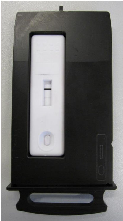
Figure 28: Position of the test cartridge in the test cartridge adapter
